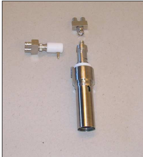
Figure 3: Typical Liquid Cell Courtesy Dielectric Products Watertown, MA
