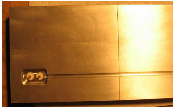
Figure 3. Alluminum Fixture for surgical electrode
