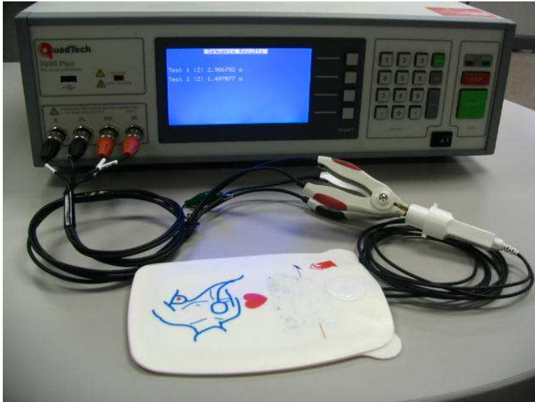
7600 Plus Connected to DF Pads
